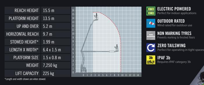
The Niftylift Height Rider 15 (HR15) has an impressive working outreach and zero tail-swing that helps it to reach awkward jobs, especially when space is limited. Its super-efficient power system allows the batteries to work for longer, so more tasks can be completed and running costs reduced.
